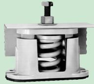
Type C spring mounts are designed so that neoprene sponge inserts limit movement during start and stop and prevent contact between the projections of the upper and lower semi-steel casting. These inserts are designed for a minimum of damping in all directions. This is a good design for engineers that prefer housed mountings.
