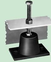
Type ND neoprene mounts are designed for both high static deflections and simplified installations. The rubber is loaded in both shear and compression to provide the desirable straight line rubber-in-shear deflection curves as well as overload protection. They are molded assemblies with skid resistant rubber ridged baseplates and need not be bolted to the floor on most installations.
